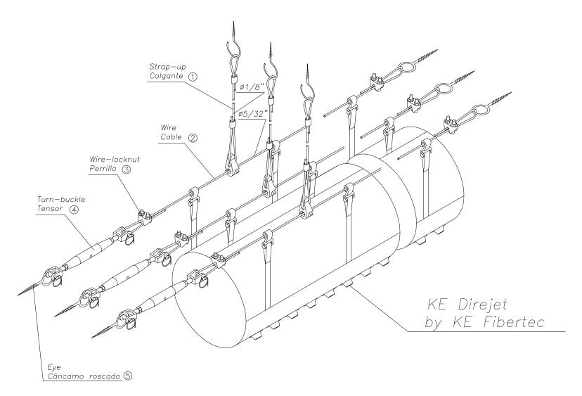
Triple Cable Suspension Detail for Fabric Ducts (12 o' clock Attachment)
