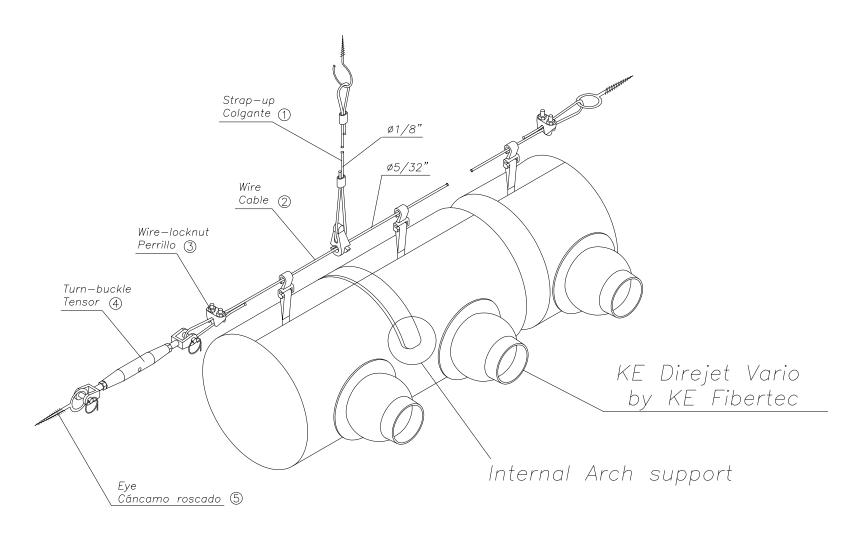
Wire Arch Suspension Detail for Fabric Ducts (12 o' clock Attachment)
